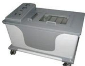
Max panel:400×400mm, it can electroplate for 5 boards at the same time, Minimum hole:0.6mm, Max thickness diameter ratio, 3:1, Output voltage:0-15V,adjustable continuously, Output current:0-20A, adjustable continuously, Dimension:420×430×420mm, With 2 groove, one is for tin-lead plating, the other is for quit tin-lead.
