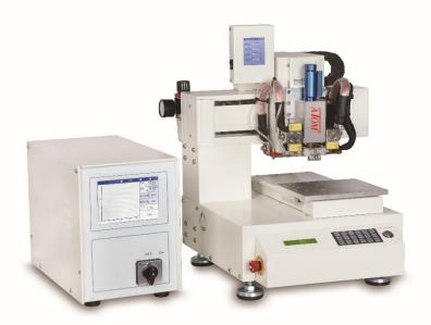
3-Axis Hot Bar Soldering Robot
