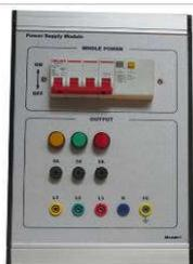
The power control unit adopts the embedded installation mode, and the 4P circuit breaker is used as the total power supply access switch of the training equipment, and it is equipped with corresponding power indicator lights and fuses.
