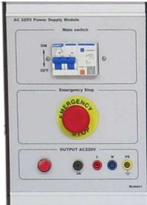
The power control module adopts the embedded installation mode, and the 2P circuit breaker is used as the total power supply switch of the training platform, and is equipped with electrical components such as emergency stop and power indicator.
